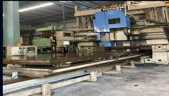
Double Colum Vertical Machining Center ( Under Commissioning ) 7000 X 2500 X2000 MM
