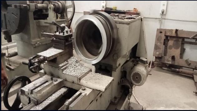
Lathe Machine OD Ø400mm X L900mm
