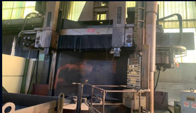
CNC VTL ( Under Commissioning ) 2500 mm Turning Dia
