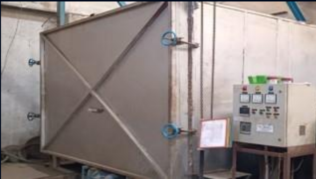
Heat Treatment Furnace 600 ° C 2600 X 2600 X 2000 MM
