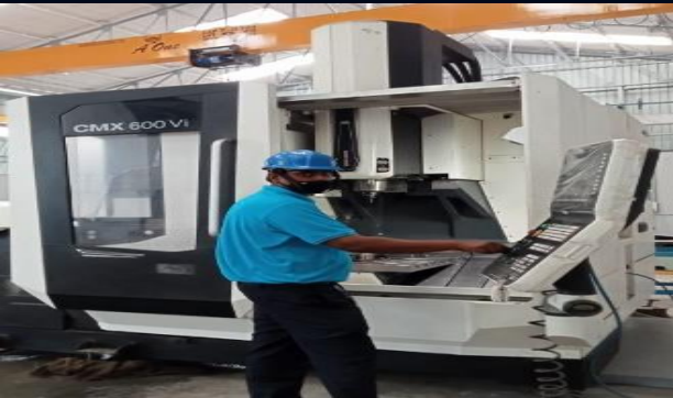
CNC Vertical Machining Centre DMG Mori X600mm X Y560mm X Z510mm
